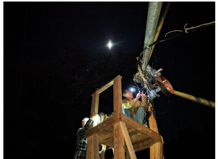
K2UYH changing feeds during the ARRL MW EME Contest. K2BMI is at the back of the platform
