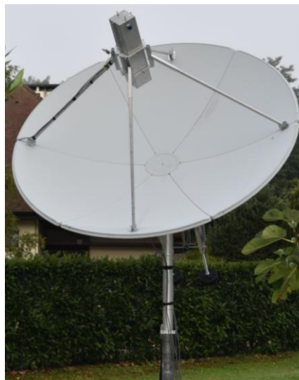
F6ETV's 2.4 m dish with 23 cm septum feed
