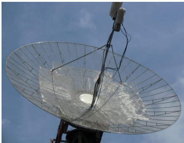
JA6XED's 5 m dish with extra screening for 3 cm
