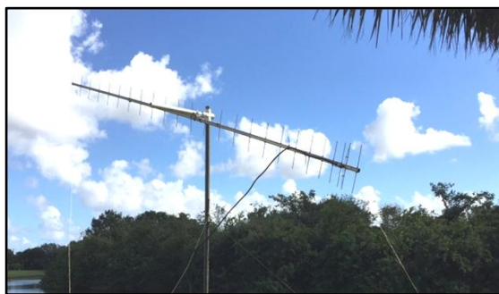
5 wl yagi used by K1DS in contest on 70 cm
