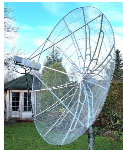
PA0TRB's new 3.5 m dish with 1296 feed
