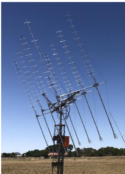
ZS4TX's 70 cm 4 x 2 yagi array with rotatable pole
