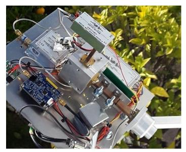
CT1BYM's 24 GHz 4W SSPA from Kuhne electronics
